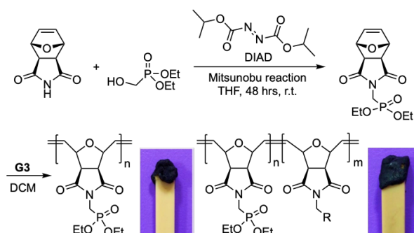
Figure 10: Flame retardant ROMP homo- and copolymers (R = benzyl, naphthyl, anthracenyl) incorporating phosphonate groups and photographs of chars from flame testing on treated polypropylene (PP) test samples. Untreated PP test pieces were completely consumed. Adapted with permission from Ref. [53]. Copyright © 2018 Wiley-VCH.
