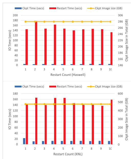
Fig. 3. Checkpoint/Restart overhead of MANA when running GROMACS with 2048 processes on Haswell (upper panel) and KNL (lower panel) nodes on Cori's Burst Buffer. The blue and red bars show the checkpoint and restart time, respectively; the yellow line indicates the total size of the checkpoint files.
