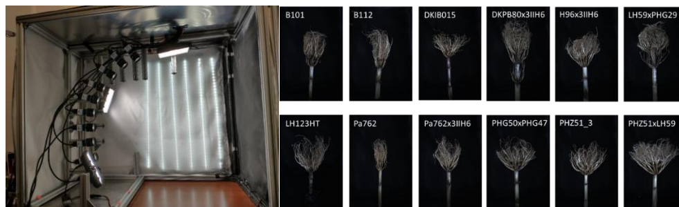
Figure 1. 3D root imaging chamber.
