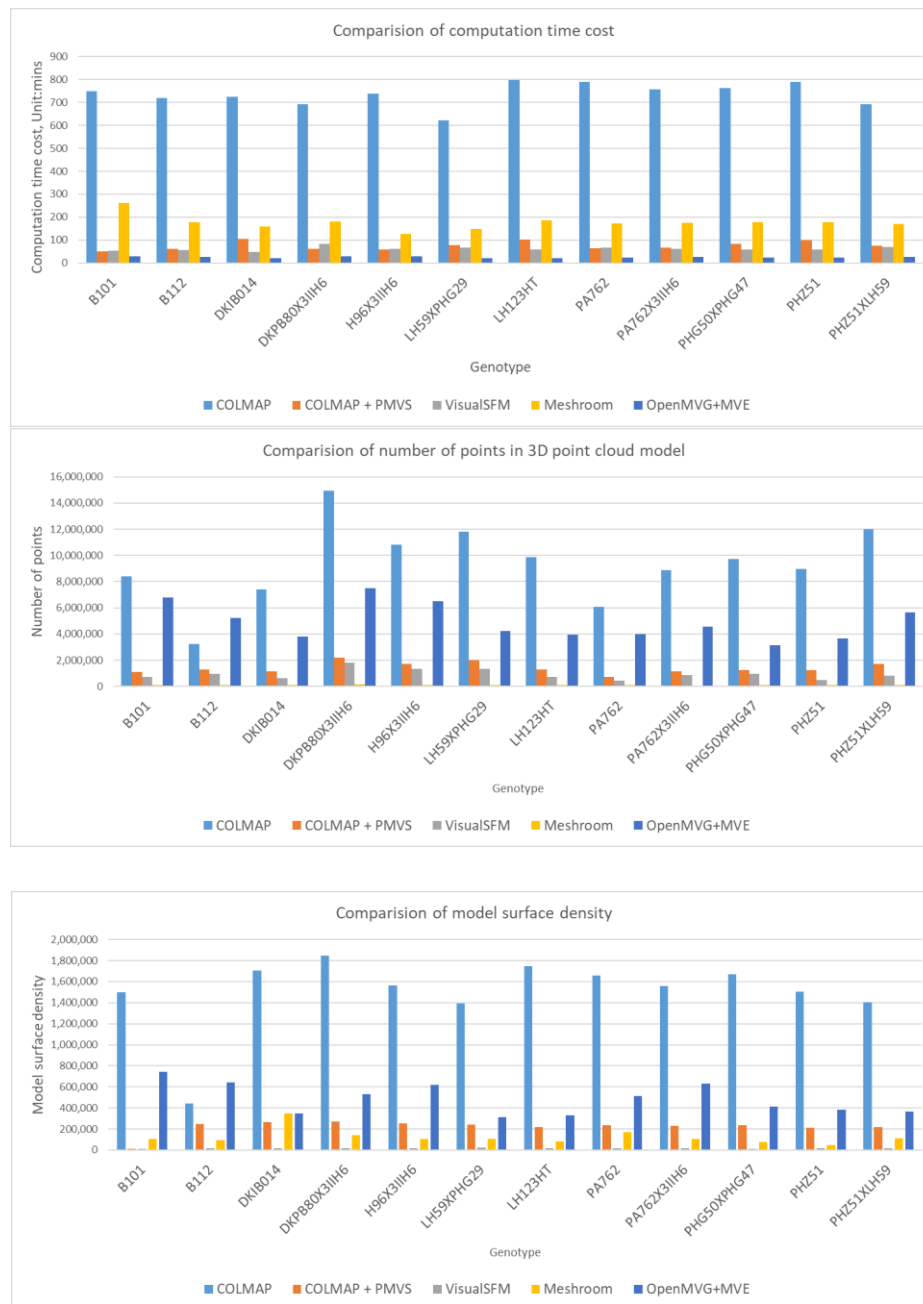
Figure 3. Comparison of time cost, number of points and surface density of 3D models
