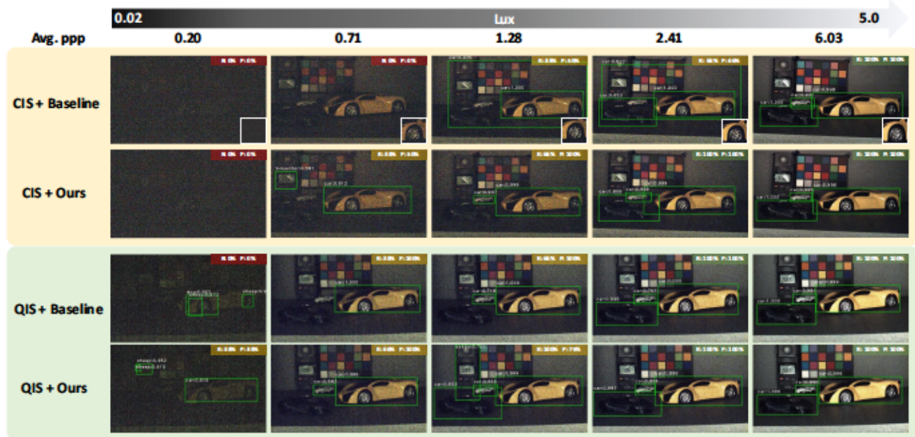
Figure 8: Comparison of different sensors and different methods on real data. The visualized figures are tone mapped and the baseline method is Faster R-CNN. We choose 5 different lux levels ranging from 0.02 to 5.0, equivalent to Avg. ppp ranging from 0.20 to 6.03. In the right-top corner of images, the recall (R) and precision (P) are computed, enclosed in frames with different colors. Red/Yellow/Green indicates totally failed/partially correct/totally correct, respectively. In the first row, we zoom into the left-front side of the yellow car and show details in the right-bottom box. We can see that in the extremely low light condition, the images suffer from the high-noise problem.
