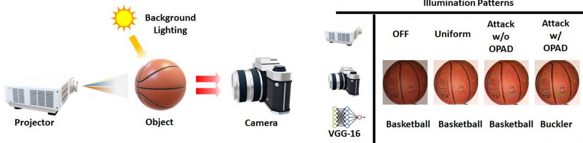
Figure 1. OPAD is a projector-camera system that uses structured illumination to perturb the appearance of objects. The four configurations shown on the right-hand side are: (1) When the projector is off, the classification remains correct. (2) Whenever we turn on the projector, it will generate a uniform illumination. Most classifiers today are robust to this kind of brightness offset. (3) If we illuminate the object with an attack pattern but do not compensate for the environment loss, the classification remains correct. (4) When we use OPAD to compensate for the loss, we successfully attack the classifier to the targeted class.
