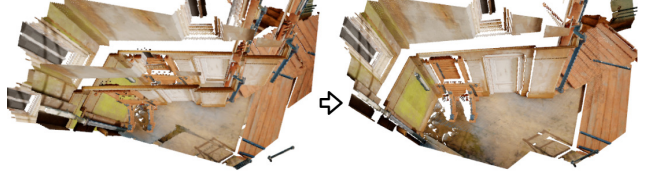
Figure 4. Example Sim3 registration, the network takes two RGB-D scans as input and predicts a similarity transformation which aligns the two scans.
