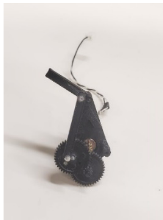
Fig. 5. In-house mechanical flapper designed to mimic the flapping amplitude of monarch butterfly in free flight.
