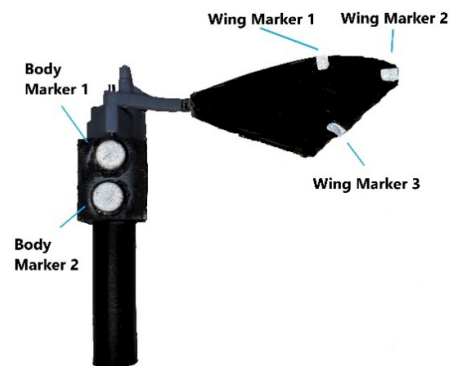
Fig. 4. The assembly of the in-house mechanical flapper and the attached monarch wing. The reflective markers used for optical measurements are labeled. The flapper and the mount are painted black to reduce camera noise.
