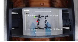
(a) Translation using Eq. 15 (b) Translation using Eq. 17 (c) Oscillating input turning (d) Rectangle tracking Fig. 9: Results from two-link swimmer (magnetization: 1:6). See supplementary videos for experiments.
