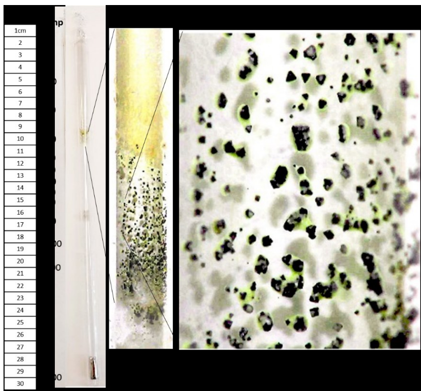
Figure 2: Silica glass tube containing I(Cl+S) glass source after cooling, with approximate temperatures of formation of primary vapor-deposited material indicated. Capsule containing the source is at bottom. Inset shows enlargements of the region in the tube containing well-formed octahedra adhered to the tube by a fine grained greenish yellow precipitate. Just below \sim 300^{\circ}\text{C} , a ring of orange fine-grained material was formed.
