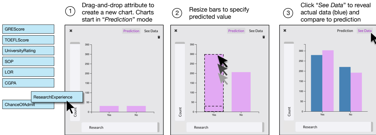
Figure 2: Illustration of the interaction sequence for specifying data expectations in a bar chart.
