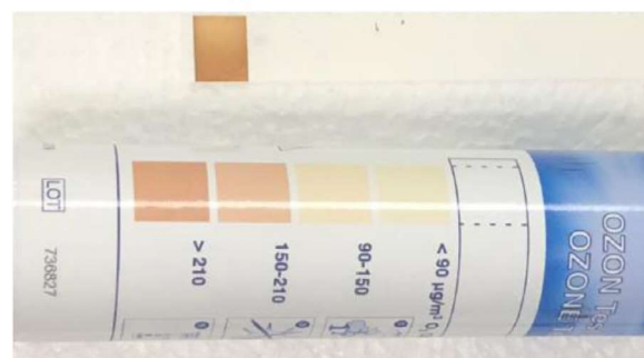
Fig. 3. Test for ozone concentration after 10 min exposition to CAPPJ. The ozone test strips (Macherey-Nagel Company, Duren, Germany), when placed under the cold He-plasma jet at a distance of 1 cm for 10 min, show production of ozone by the He-plasma jet in a concentration of 210 \mu\text{g}/\text{m}^3 or more. Temperature was 20 °C.
