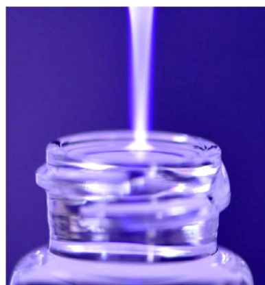
Fig. 2. Schematic diagram of CAPPJ treatment of water surface. (Left) Cold He-plasma jet and (Right) photo of the air/water interface in a contact with the He-plasma jet. 20 ml clear borosilicate glass vials with dimensions of 27 mm x 58 mm were used in all experiments with CAPPJ treatments. The diameter of the water surface was 15 mm. The temperature was 20 °C.
