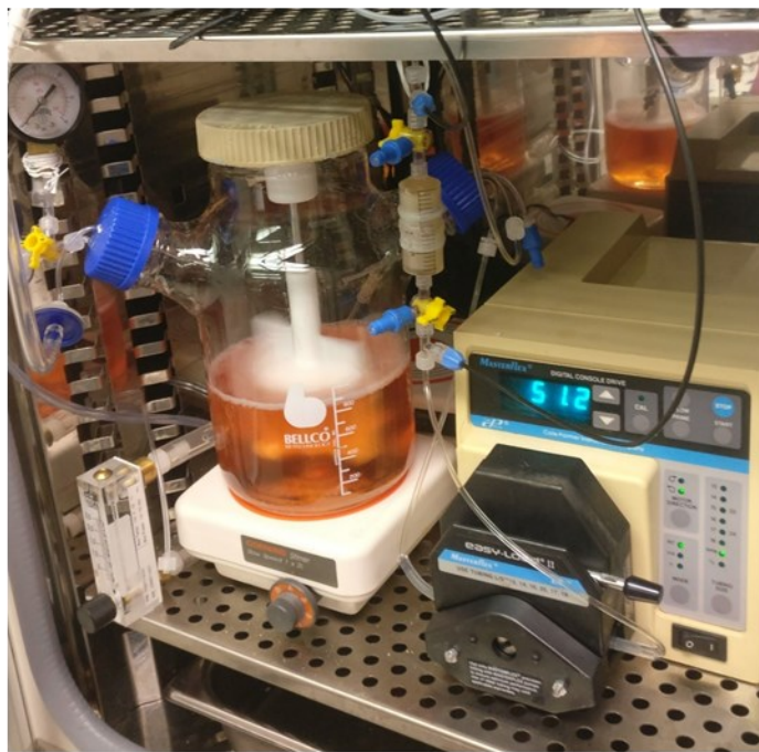
Supplementary Figure S1. (a) Detailed configuration of a RS bioreactor. (b) The RS bioreactor in a CO 2 incubator.
