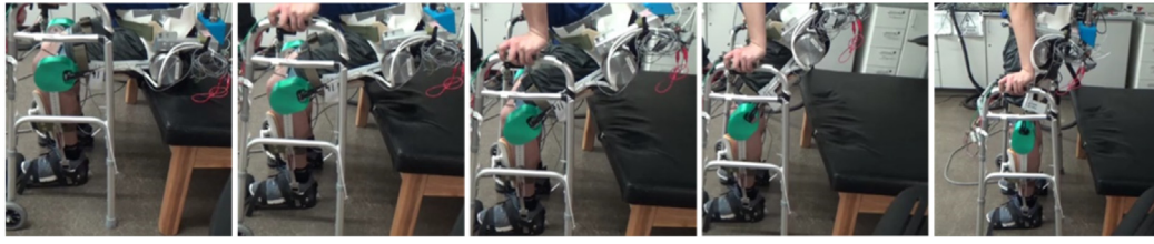
Fig. 3. The experiment record of able-bodied human sitting-to-standings with assistance from the wearable robotic system.
