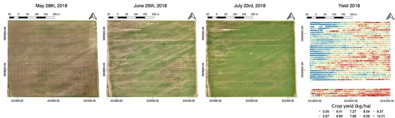
Figure 3. Time-lapse of UAV-RGB image acquired during the growing season (May 28th, June 25th, and July 23rd), and the point-cloud maps of the yield (kg/ha) acquired by the combine harvester (right figure). Maps made with QGIS (v 3.6, https://www.qgis.org ) 36 .
