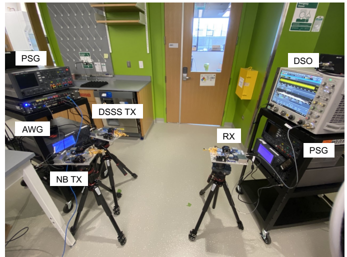
Fig. 3. The experimental set-up consisting the AWG, two transmitters (one transmitting a DSSS signal and the other a NB signal), one receiver, and the DSO.
