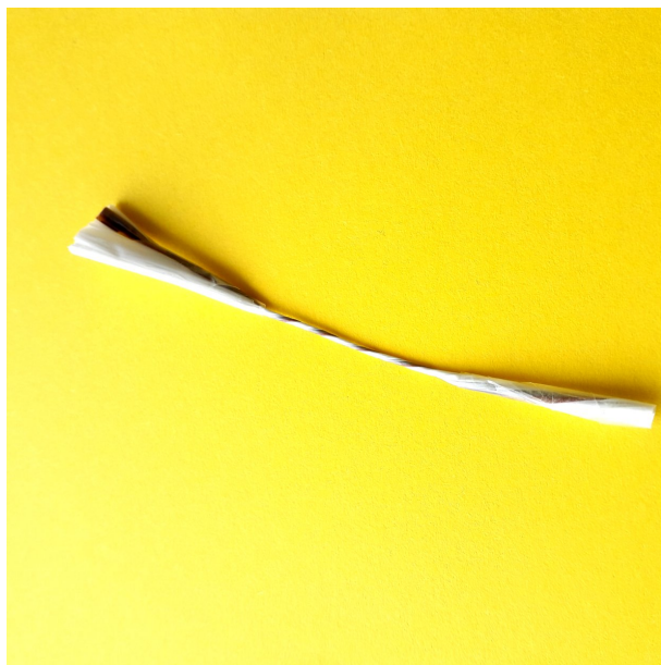
Figure S3: Scrolled yarn fabrication. A scrolled yarn with fans made by twist scrolling a polyethylene sheet held at the opposite ends where fans develop. The twisted yarn structure is heat treated to freeze in the twist.
