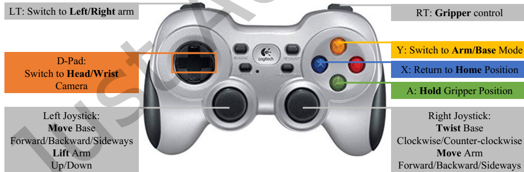
Fig. 3. Gamepad controller configuration for teleoperation interface.
