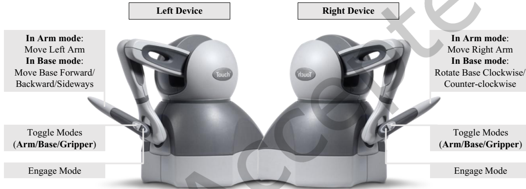
Fig. 4. Stylus device (Geomagic Touch) configuration for teleoperation interface.
