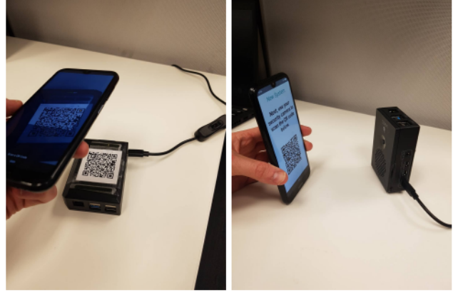
Fig. 3. Establishment of a secure and authenticated Bluetooth pairing to setup CaTUs by scanning QR codes (visual channel).
