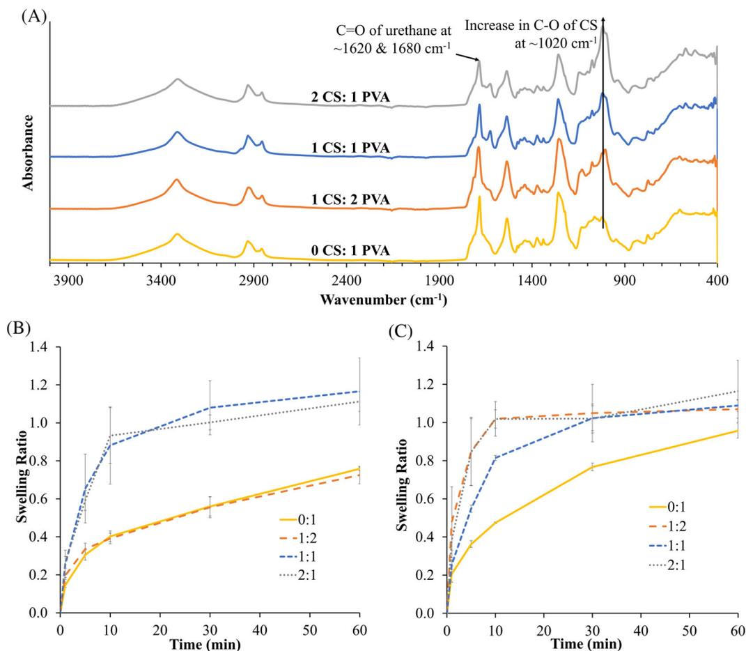
**FIGURE 3** (A) Fourier transform infrared spectra of poly(vinyl alcohol) (PVA) 6k hydrogels with varied cornstarch content. Swelling profiles of (B) PVA 6k and (C) PVA 25k hydrogel films in water at 37°C. Mean  $\pm$  standard deviation displayed ( $n = 3$ )
