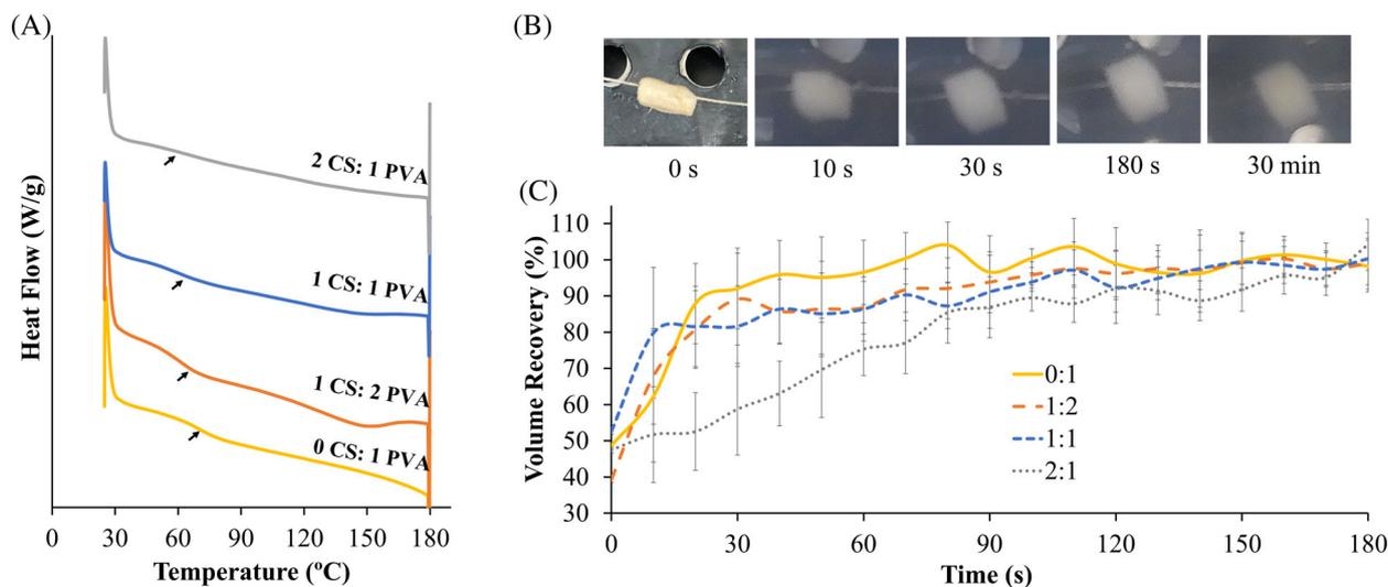
**FIGURE 6** Thermal and shape memory properties of hydrogel foams. (A) Differential scanning calorimetry traces of PVA 6k foams. Arrows denote endotherms associated with glass transition ( $\sim 60\text{--}85^\circ\text{C}$ ) temperatures ( $T_g$ ). (B) Representative images of volume recovery of 0 CS:1 PVA 6k foam. (C) Volume recovery profiles of PVA 25k formulations ( $n = 3$ ). CS, cornstarch; PVA, poly(vinyl alcohol)
