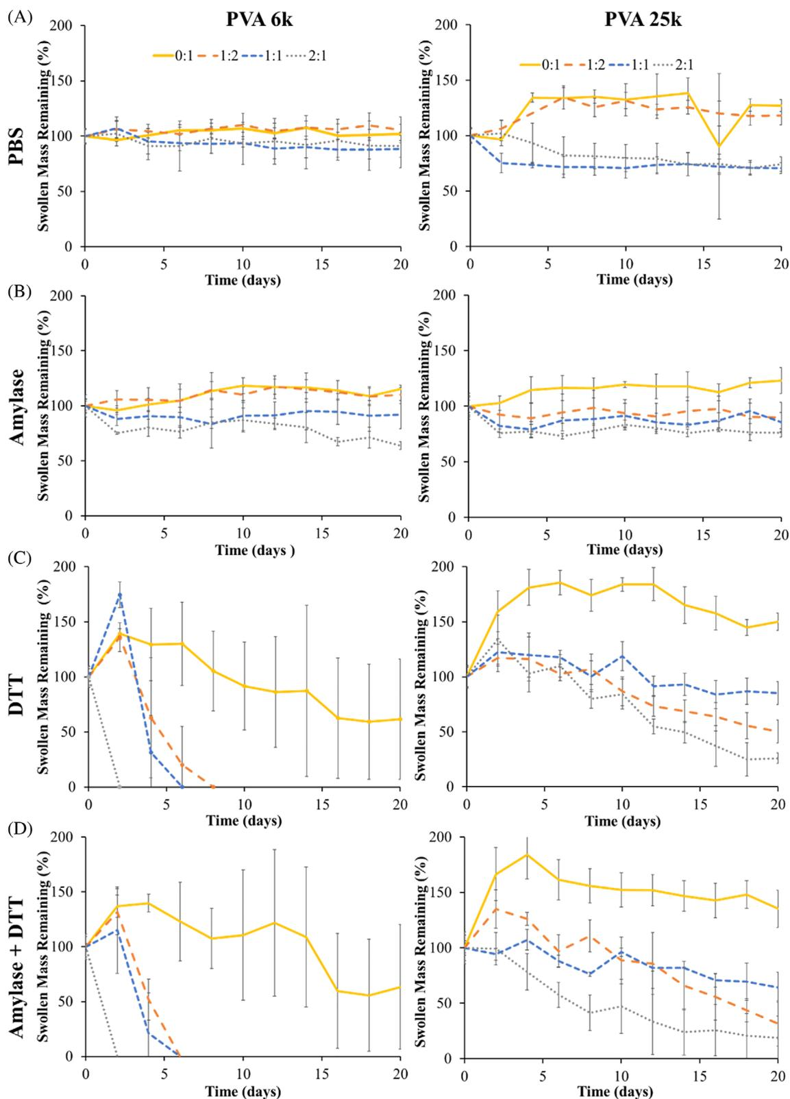
**FIGURE 7** Degradation profiles (swollen mass remaining) in (A) PBS, (B) 100 U/ml amylase, (C) 10 mM DTT, and (D) 100 U/ml amylase + 10 mM DTT of (left) PVA 6k and (right) PVA 25k hydrogel foams ( $n = 3$ ) DTT, dithiothreitol; PBS, phosphate buffered saline; PVA, poly(vinyl alcohol)
