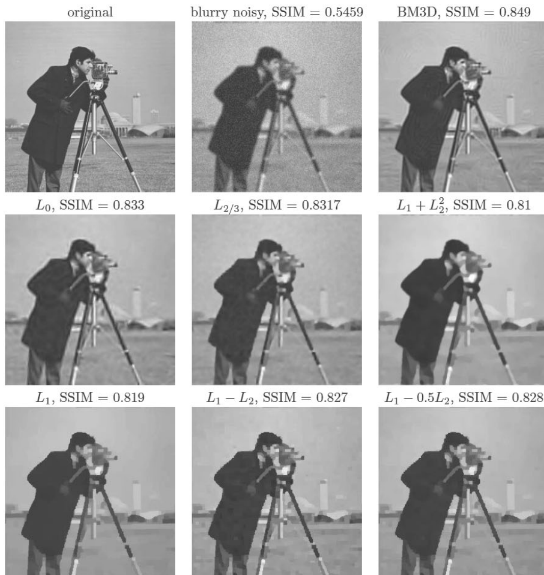
Figure 13. Deblurring results with comparison to L_0 in [34], L_p for p = 2/3 in [25], L_1 + L_2^2 in [2], and the state-of-the-art deblurring method BM3D [13].
