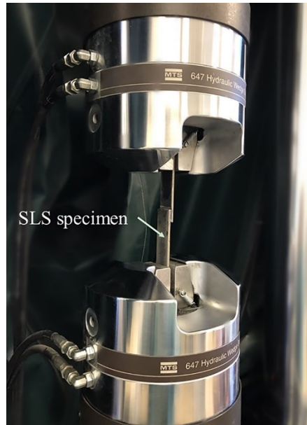
Fig. 2. The SLS test setup
