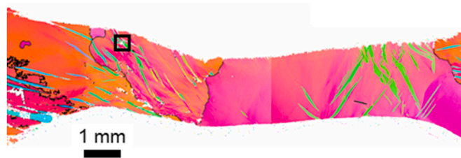
Fig. A2. Location of ROI depicted in Fig. 7 (sample 4 at a strain of 0.1). Note that the straight dividing lines sometime occurring in the maps are an artifact of stitching of separate IPFs taken with some detector distortion commonly occurring at low magnification.
