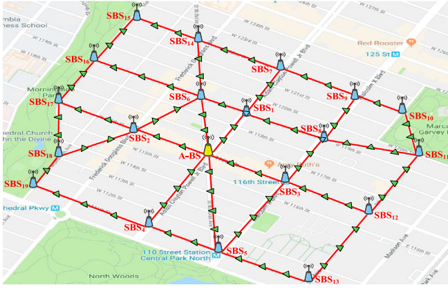
Fig. 1. Relay-assisted mmWave backhaul network in a section of Manhattan.
