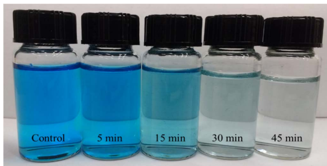
Fig. 4. Samples treated at 8 kV, 10 kHz, 1 \mu s, and 2 slm for 0, 5, 15, 30, and 45 min showed the steady degradation of MB dye.
