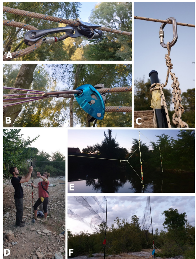
Fig. 2 - Photos of the skynet as trialled by the authors. A. Use of a Petzl basic as the rope grab in a 3:1 haul system to tension the TL. B. Petzl gri gri used to remove slack and maintain tension on one side of the TL, attached to the tree behind via a carabiner and nylon climbing sling. C. Knotwork attaching a pole to TL. Clove hitch secures guy rope to pole; carabiner is clipped to TL and through a figure-of-8 on the bight. D. Surveyors attaching a pole to tension line. E. Suspended net in position over the pond. F. Orientation of suspended and terrestrial nets.
