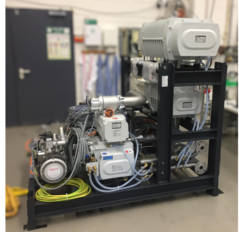
Figure 12: Photograph of the pumping station after its delivery. It consists of three roots pumps, a screw pump, two scroll pumps, a turbomolecular pump (not shown) and a gas cooler. The pumps as well as the valves are controlled remotely. Temperature and pressure sensors provide continuous readout of relevant parameters. Most of the pumps are powered using external frequency converters (not shown). Cooling is mainly performed using a common water cooling circuit.
