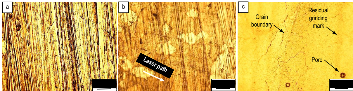
Figure 13: Evolution of surface polishing on L-PBF sample (a) ground surface, (b) partially polished surface, and (c) 0.45µm Ra polished surface. ECP at 1.2 A/mm 2 , 180s, 75% duty cycle.
