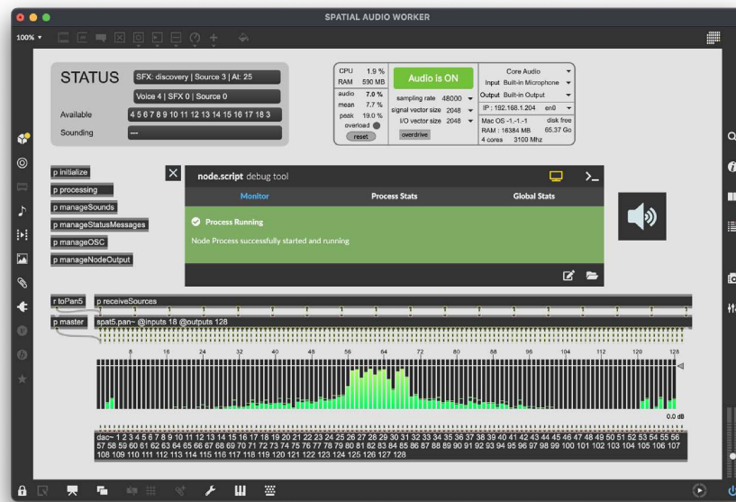
Fig. 5: The Spatial Audio Worker receives incoming audio files and their respective position information to dynamically spatialize user content. The Worker incorporates a Node.js server with an API which allows it to receive data from various applications and interfaces. One such demonstrated interface allows users to transmit audio files and manipulate their position from a browser on a personal device.
