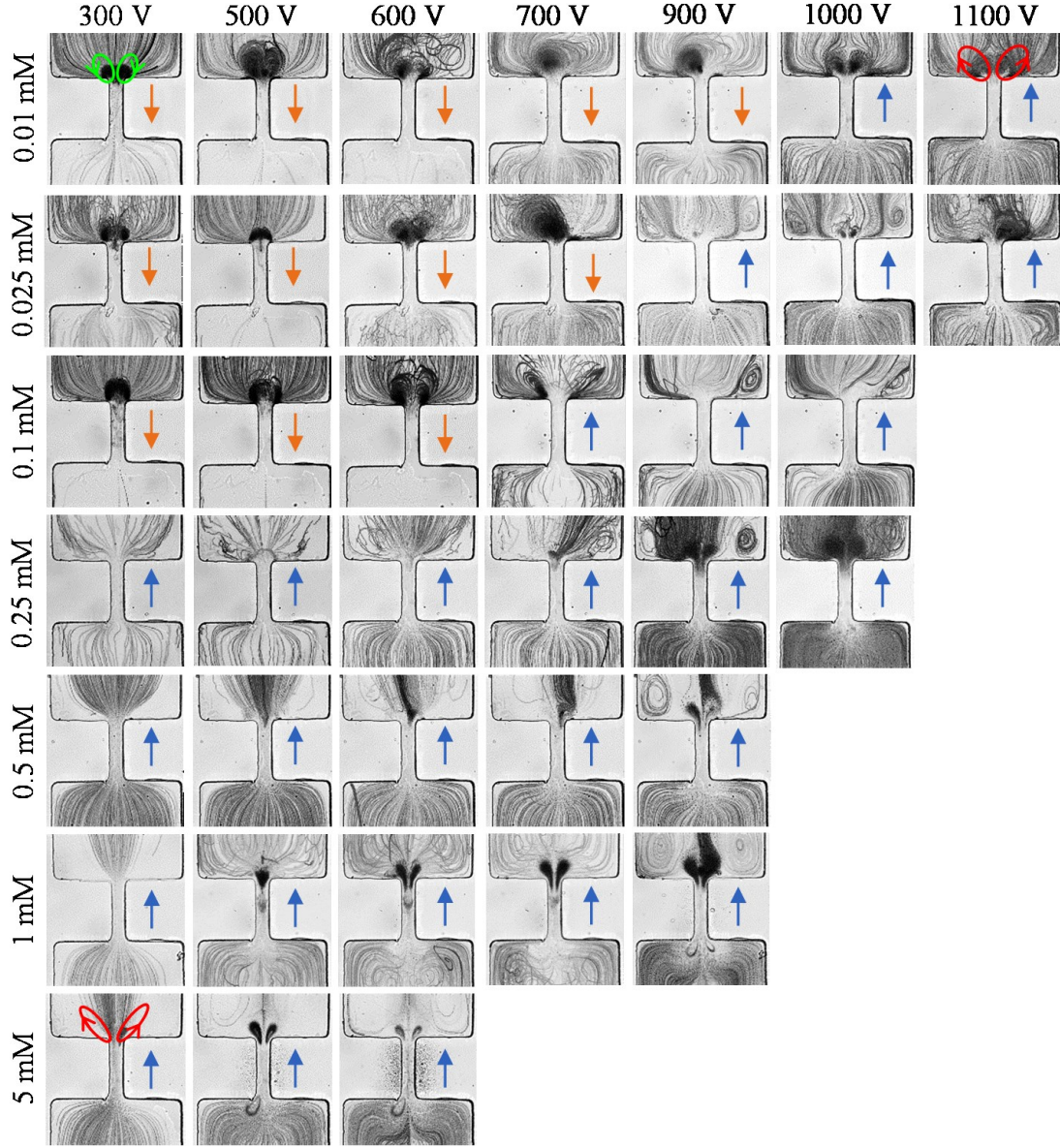
FIG. 2. Experimental images of tracing particles in a constricted microchannel in buffer solutions of different concentrations under different AC voltages. The DC voltage was fixed at 20 V and applied downwards. The arrow on each image indicates the particle moving direction inside the constriction, which switches from along the DC electric field (top to bottom) to against it with the increase of buffer concentration or AC voltage. The looped arrows on the top-left image highlight the fluid circulations of ICEO while those on both the top-right and bottom-left images highlight the fluid circulations of ETF.
