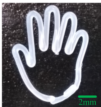
Figure 6. Thermoplastic PCL 15 -PβMδVL-PCL 15 was printed to a hand-shaped structure through fused deposition modeling (FDM) at 60 °C.
