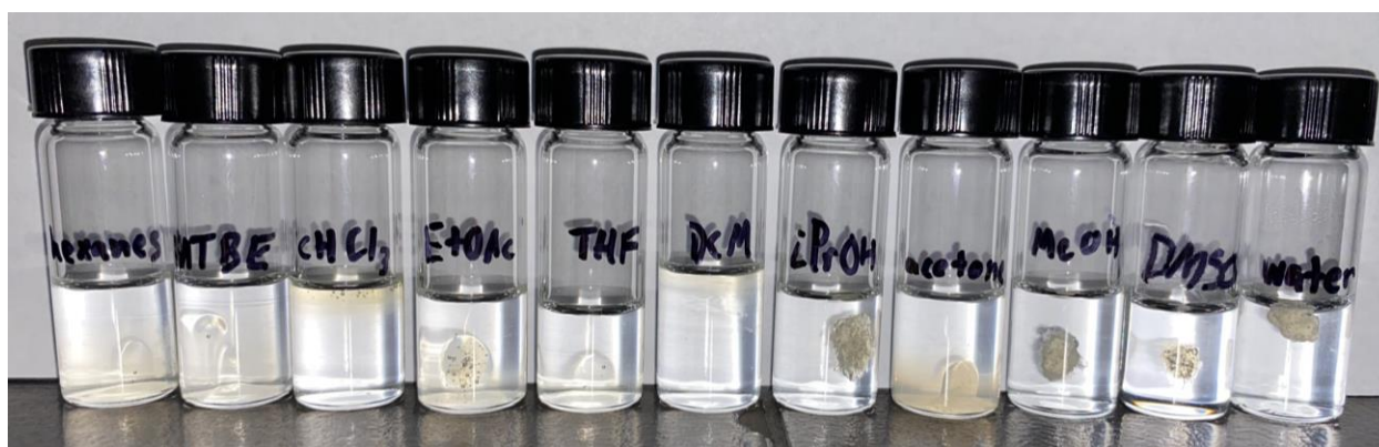
Figure 29. Swelling tests of 20–30 mg of cross-linked poly(myrcene-co-dibutyl itaconate) after ~60 min in a variety of solvents ordered from left to right by ascending dielectric constant. Adapted from Ref. 289. Copyright 2016 American Chemical Society.
