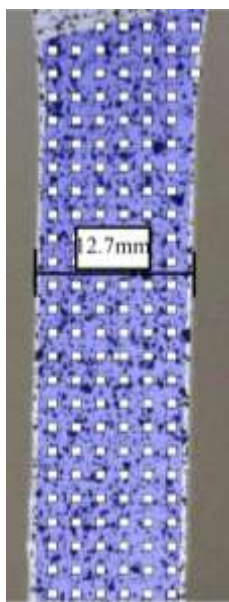
Figure II. Example of spacing of the points where GOM correlate reported strain values for the reference image of the CTBN50% 500kg sample 1.
