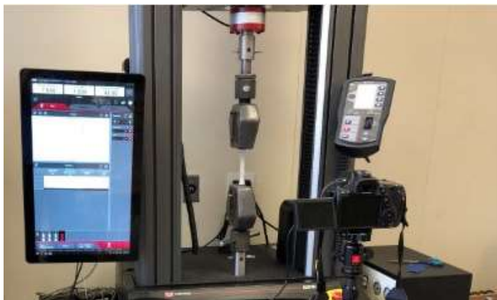
Figure I. DIC and tensile test setup.
