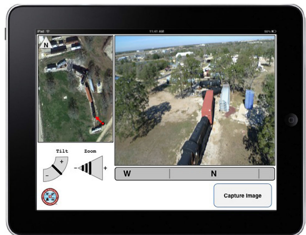
Fig. 5 Refined Implementation of the Mission Specialist Interface on an Apple® iPad Used in the Experimental Study. A Captured Image of the Simulated Train Derailment is Shown in the Video Display Window. The Mission Specialist Controls the Payload Camera and Captures Images in the Same Manner as the Initial Implementation in Peschel and Murphy [16]. Role-Specific Information Was Added that Included an Overview Map with UAV Position and Heading, a Digital Compass, and Payload Camera Tilt and Zoom Indicators (Courtesy of Center for Robot-Assisted Search and Rescue)
