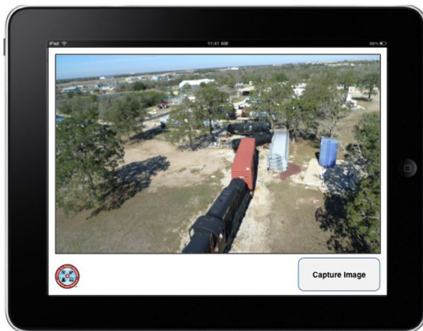
Fig. 4 Initial Implementation of the Mission Specialist Interface on an Apple® iPad Used in the Exploratory Study by Peschel and Murphy [16]. A Captured Image of the Simulated Train Derailment is Shown in the Video Display Window. The Mission Specialist Swipes (Up and Down) and Pinches (In and Out) Directly on the Video Display to Control the Payload Camera for Tilt (Up and Down) and Zoom (Out and In). Images are Captured by Pressing the Capture Image Button (Courtesy of Center for Robot-Assisted Search and Rescue)
