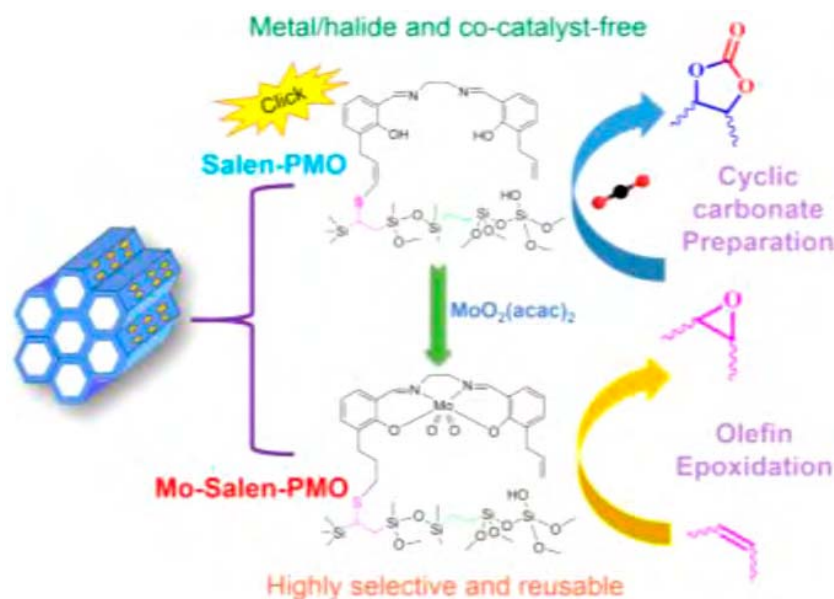
Figure 14. Examples of organocatalysts, salen ligands with or without Mo ions, tethered to the surface of a periodic mesoporous organosilica (PMO). 188 Reproduced with permission from ref 188. Copyright 2021 Wiley-VCH GmbH.
