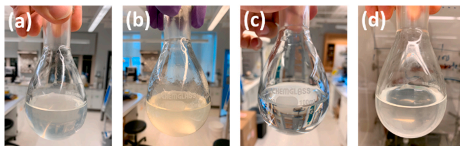
Fig. 1. The dispersed phase containing NAC/gum/surfactant in water and EC in EtOAc, is used in the IPS process. (a) sample I2, (b) sample I7, (c) sample I11, and (d) sample I15. See Table 1 for the reaction formulations and conditions.
