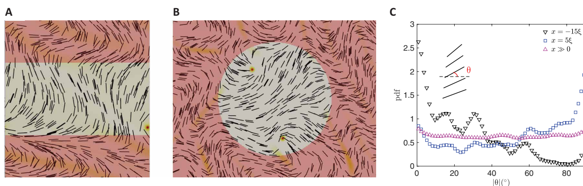
Fig. 2. Anchoring effect at activity gradient boundary. (A) A slab of passive region of width 100 bound by active regions at activity level \alpha = 0.002 . (B) A passive circular region with diameter 160 surrounded by active region exhibiting two +1/2 defects, reminiscent of a passive nematic confined in a cylinder with homeotropic anchoring. (C) Probability distribution function (pdf) of director orientations at various positions relative to the activity boundary ( x < 0 , passive region; x > 0 , active region), showing the emergence of a homeotropic anchoring effect at the passive side of the boundary.
