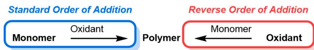
Figure 2. Differences between standard and reverse addition in chemical oxidative polymerization.
