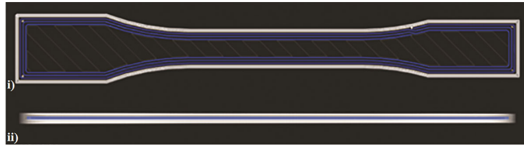
Figure 1. Top and side views of ASTM D638 Type 1 CCFRAM tensile specimen. (a) blue color denoting continuous carbon fiber reinforcement strands. (b) Top view (i) denoting number of rings, side view (ii) denoting number of layers. (c) Developed using Markforged Eiger ® slicing software.
