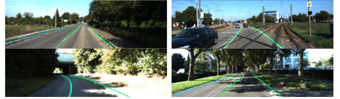
Fig. 12: Sample results of our method when applied to the KITTI dataset where the green curves indicate the ego-lane boundaries.
