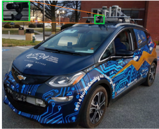
Fig. 7: Test vehicle - GM Chevy Bolt EV equipped with a color camera mounted on the roof of the vehicle and other sensors.
