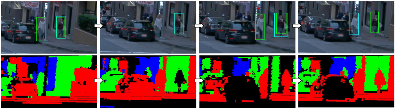
Fig. 5: Robust pedestrians tracking: In the top row, there are two pedestrians detected in the first frame and then in the second frame model failed to detect one of the pedestrians. However, in the next two consecutive frames that pedestrian is detected and tracked again which represents the robustness of our method. The green and cyan bounding boxes in the top row represent detected and tracked pedestrians, respectively. On the other hand, the bottom row shows the corresponding LiDAR scans where the relative distance of objects from the ego vehicle is shown by a jet color spectrum.
