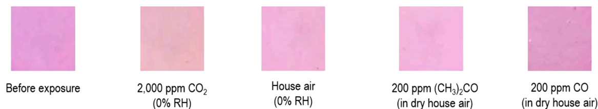
Fig. 4. PSP-ED/ZIF-8 profiles before target gas exposure; exposed to 2000 ppm carbon dioxide (dry); dry house air; 200 ppm acetone (in dry air); and 200 ppm carbon monoxide (in dry air).
