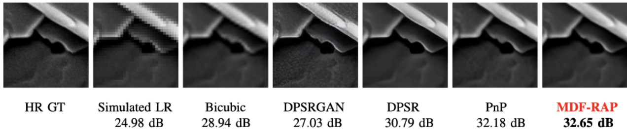
Fig. 5. 4x super-resolution reconstructions of a simulated LR EM image of pentacene crystals with \mu = 0.8 for MDF-RAP. Each shows a zoomed field of view 5.34 \mu wide. MDF-RAP performs well in terms of PSNR (and FRC in Fig. 8) while DPSR produces edges that are even sharper than the edges in the HR GT.
