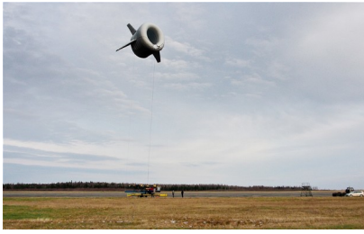
(a) Altaeros Buoyant Airborne Turbine (BAT) [11]
