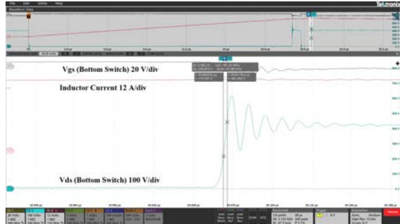
Fig. 13. Turn OFF dV/dt for DPT at 400 V 55 A.
