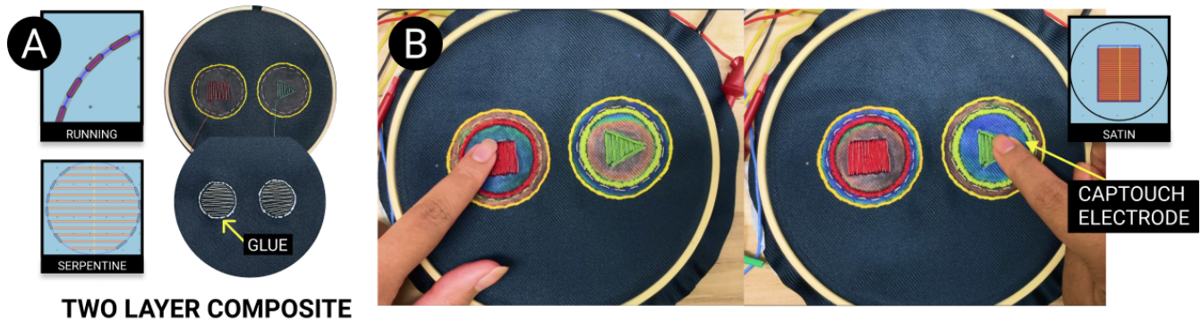
Figure 8: Play/Stop Textile User Interface. A) an LCTD is constructed by gluing two fabric layers, each with a high-power density embroidered heater; the glue and reinforcing satin stitch border are used as thermal barriers to isolate heat to each heater’s respective regions. B) A user activates the satin stitch capacitive touch electrode in the center of each button through touch; a halo region around each button indicates available actions whereas the inner button region indicates current state.
