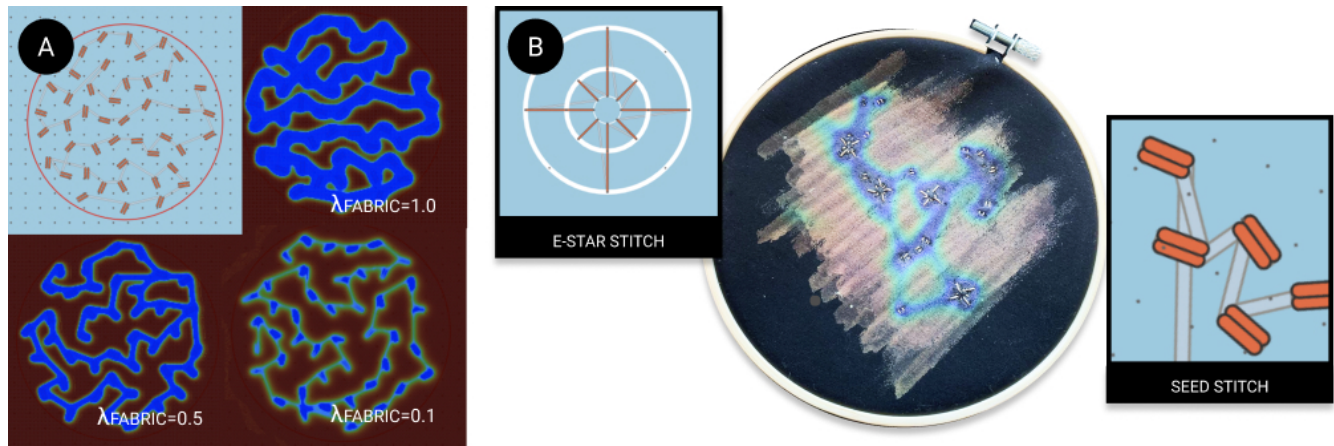
Figure 9: Orion’s Belt. A) A seed stitch heat transfer simulation is run with different fabric thermal conductivity values; B) a seed and star stitch is used on a thick fabric along the points of the Orion’s Belt constellation — when powered, the connected constellation becomes visible in the liquid crystal display.
