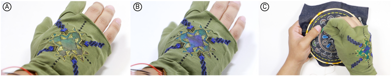
Figure 11: The Embellisher's Glove. A) A simplified glove design is controlled from an external power controller worn on the wrist; a silicone balloon with water forms a barrier between the user's hand and the glove, preventing body heat from activating the LCTD; B) the LCTD activated using a serpentine stitch; C) the glove cycles through its thermal expression as the embellisher works on an embroidery design, serving as a calming ambient display.
