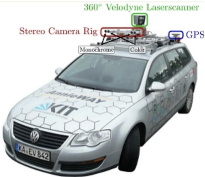
Fig. 3. AnnieWAY car used to collect the KITTI dataset[12]
