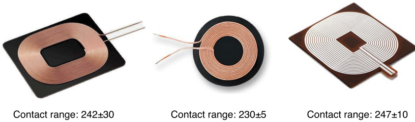
Fig. 7. Heterogeneous power receiver coils. The size and shape of the coils result in different contact range mean and standard deviation.
