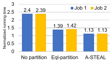
Figure 10: Adaptive scheduling. We run two jobs at the same time with three schedulers (horizontal axis): (1) No partition where each job occupies all cores, and so every core has two jobs running; (2) Eql-partition where each job exclusively uses half of number of cores in system; (3) A-STEAL where each job gets cores on demand according to its runtime parallelism (our scheduler).
