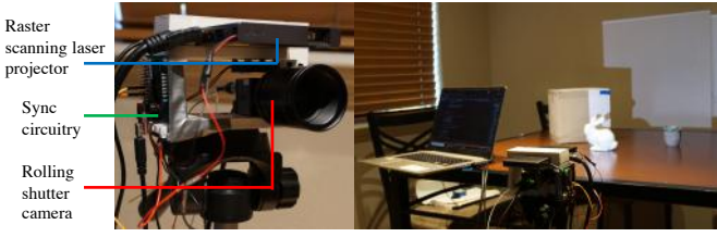
Fig. 2: Our hardware prototype for the slope disparity gating system. This synchronized projector-camera system allows for optical gating of photons from selective regions in the scene. On the right is an example scene being captured in the lab.
