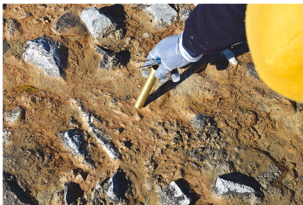
Figure 7. A photo of an investigator sampling orange mat using a cork borer. Photo courtesy of MRS.
